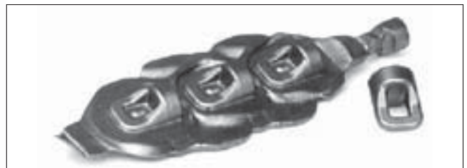
Figure 1. Typical hot forging produced on a hammer. Three components are produced in the single platter. One of the final forgings after trimming is shown on the right.
