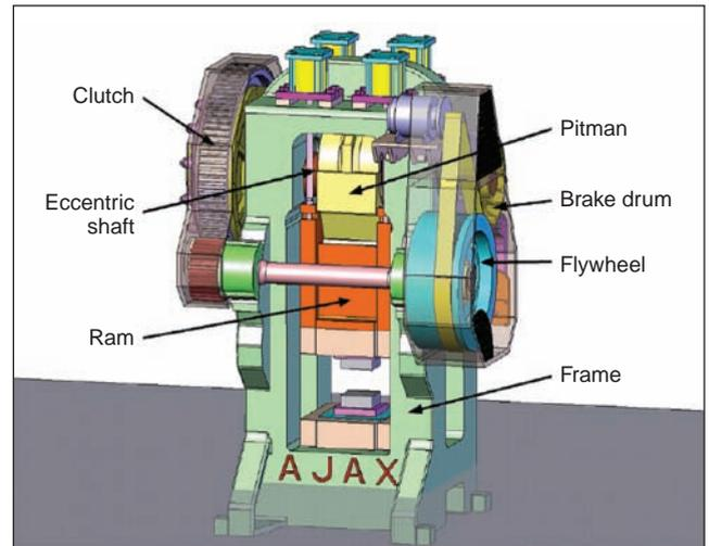
Figure 2. Schematic overview of a mechanical press, with the major components labeled
