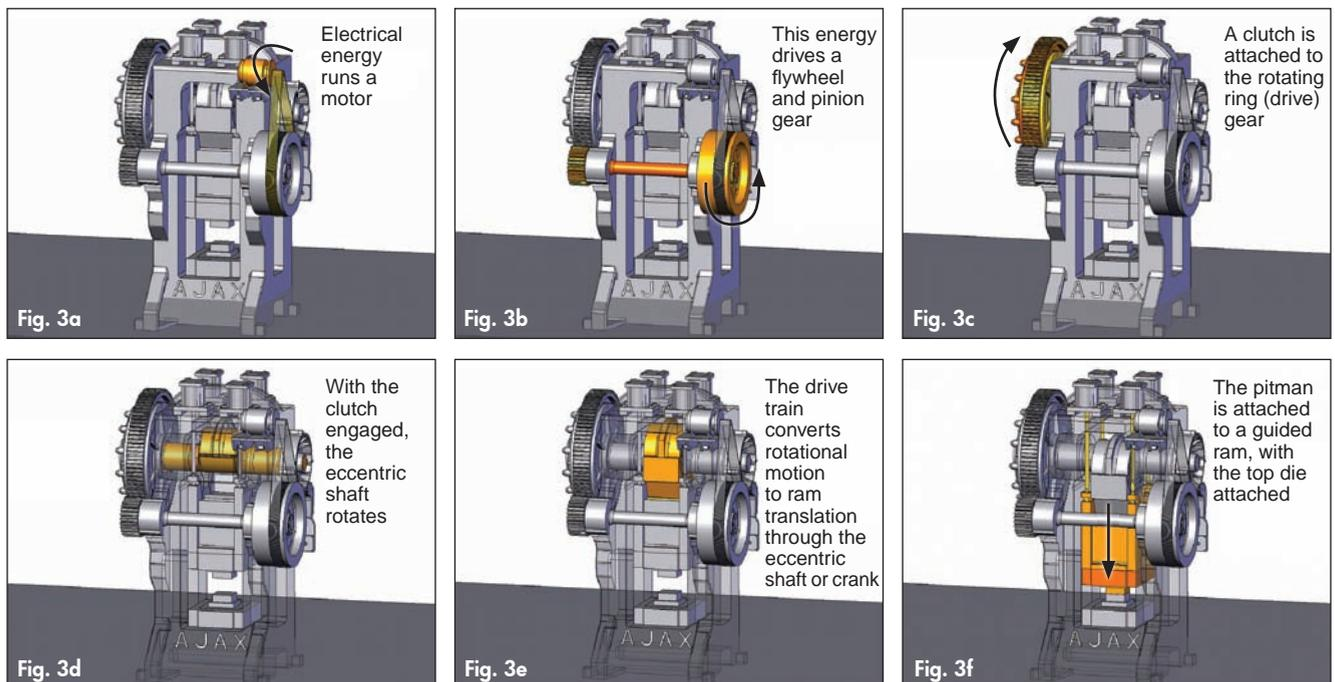
Figure 3. Operational features of a mechanical press
