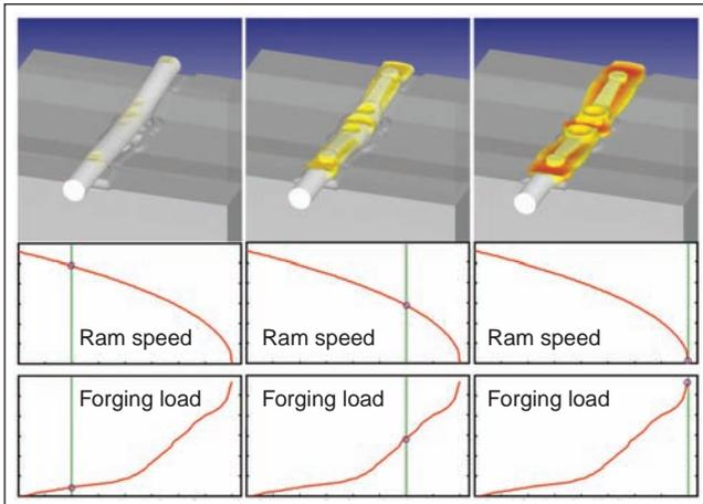
**Figure 4. Simulation of a mechanical press forging with the ram speed and forging load indicated. The simulation is shown at the very end of the stroke when the load is the highest and the die cavity is filling. Note that the ram speed is slowing down until it comes to a stop at bottom dead center. The forging load increases at the first point of contact between the die and the workpiece.**
