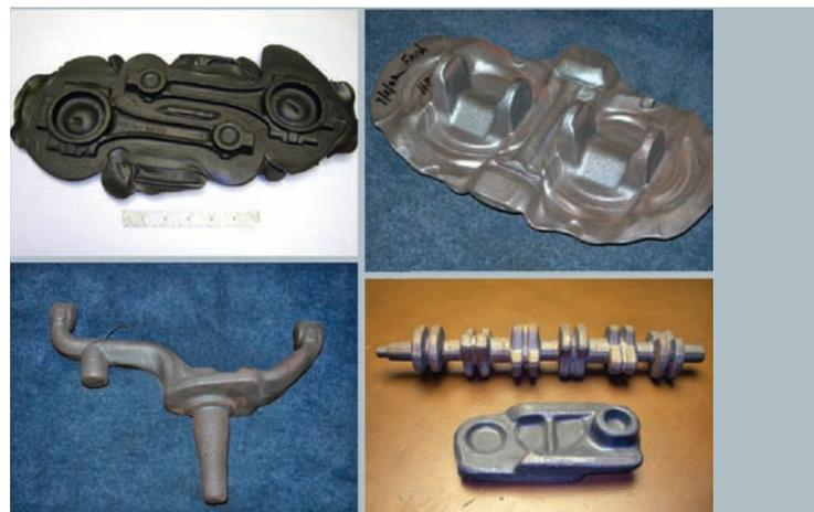
Figure 1. Typical hot-forged parts produced on a mechanical press, which can also be used for cold forging and coining operations.
